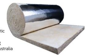
**ECOWOOL** CondenBreak blanket is designed to be used in both residential and commercial metal or tile roof systems, and under concrete slabs/soffits. The blanket dramatically slows the transfer of heat into and out of your home while also absorbing outside noise, while the reflective foil shields against radiant heat from entering the roof cavity and also controls condensation.
